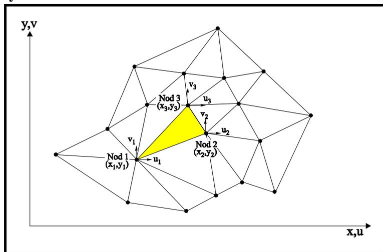
Fig.4. The discretization in finite elements of a plane structure (according to Mocanu, 1977)
