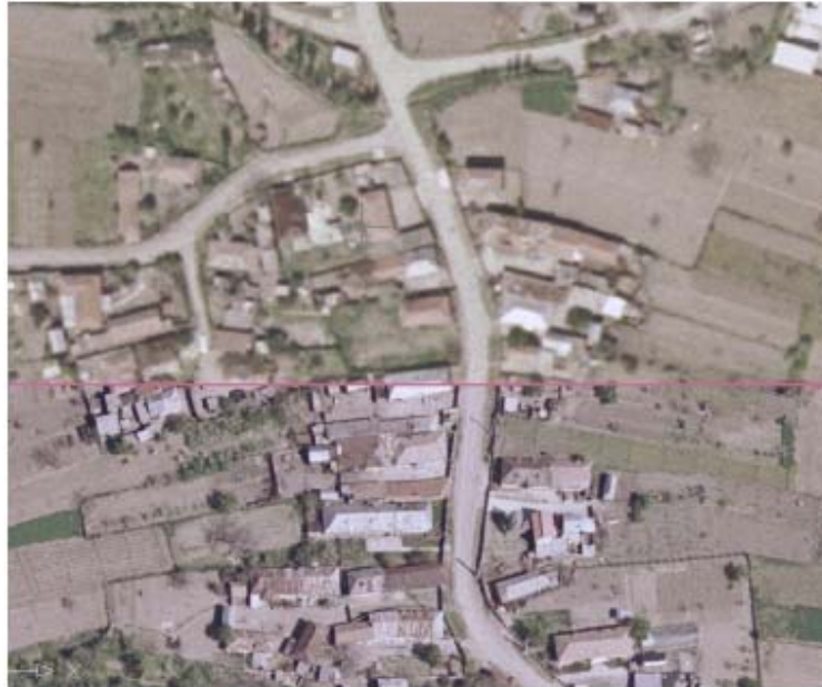
[ Fig.1 – Joining the 1:2000 and 1:5000 ortho-photograms ]
