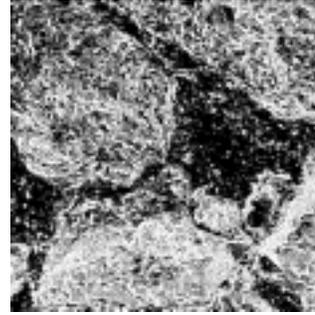
Fig. 14 Remaining points after filtering with RASCOR (white) 49.95% points removed for Inzell
