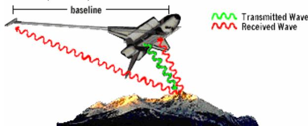
Fig. 2 Radar signals being transmitted and received in the SRTM mission
