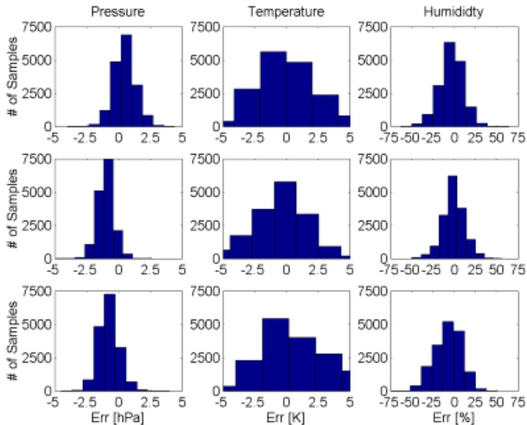
Fig 3. Histograms of the GDAS NWM-extracted and in situ meteorological parameters (pressure, temperature and relative humidity) for three of test stations: BACA (up), BAIA (middle) and DEVA (down)
