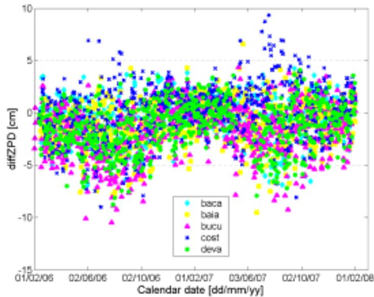
Fig 4. The GDAS NWM ZPD differences with respect to EUREF ZPD solutions for the Romanian EUREF GNSS test stations, only one (0-h UT) epoch is used for each day during the interval February 2006 - February 2008
