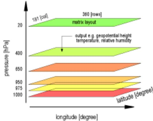
Fig 2. Data representation in the Global Data Assimilation System (GDAS) numerical weather model (NWM)
