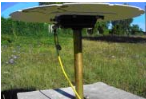
Fig.10 Forced centering system of the antenna
