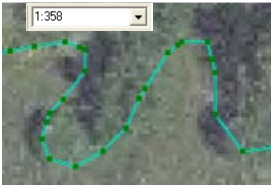
Figure 12: Example of the vertices that are located under 1 meter one of another . The scale of the digitization is 1: 1000 and the resolution of the orthophotoimage is 0.50 meter.
