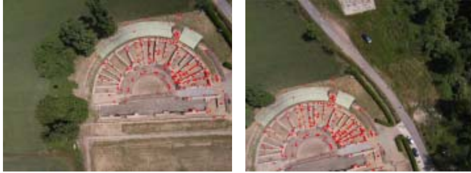
Fig. 4. Photogrammetric survey of the Theatre ruins of Benevagienna. Image correspondences automatically matched by SIFT (298 points, Th_{key}=0.0005 , L=15 ).
