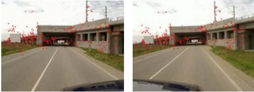
Fig. 7. Homologous points automatically extracted on a stereopair acquired by the MMS.
