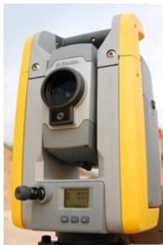
Fig. 1. The Trimble S6 Total Station and some technical details
