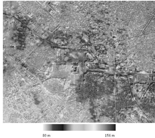
Fig. 4. ERS TANDEM DSM – 25 m resolution, generated based on ERS data (© ESA 2009)
