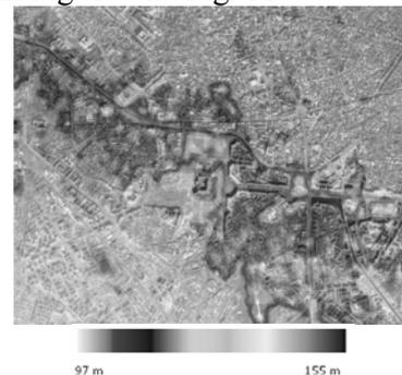
Fig. 2. SPOT 3D DSM (© SPOT IMAGE 2007) – 22 m resolution
