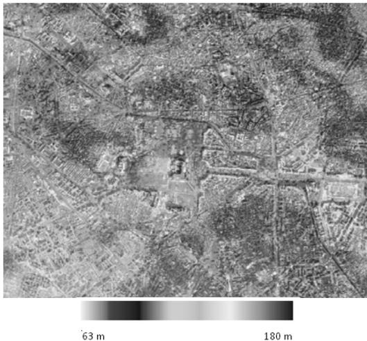
Fig. 7. TSX HS DSM - 5 m resolution, generated from TSX HS data (© DLR 2008)
