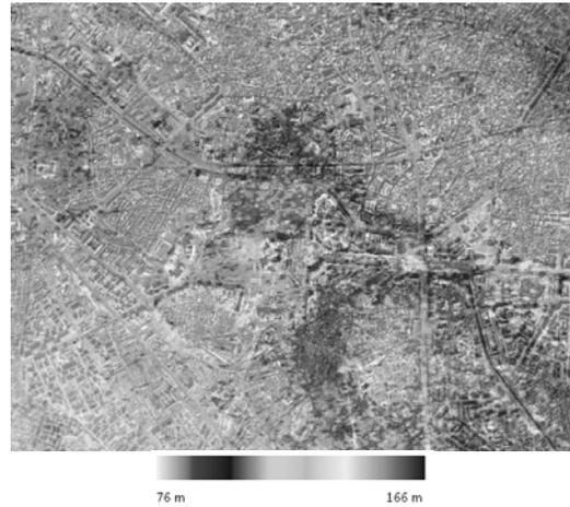
Fig. 6. TSX SM DSM - 12 m resolution, generated from TSX SM data (© DLR 2008)
