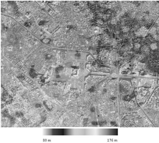
Fig. 5. ENVISAT DSM – 25 m resolution, generated from ENVISAT data (© ESA 2009)
