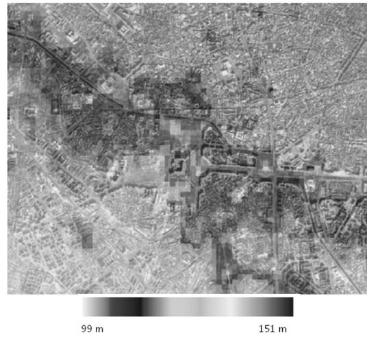
Fig. 8. SRTM DSM – 71 m resolution (© Jarvis A., H. Reuter, A. Nelson, E. Guevara\*)
