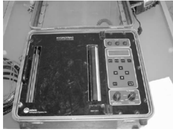
Figure. 7 ODOM HYDROGRAPHICS, HYDROTRACK type hydrographical probe
