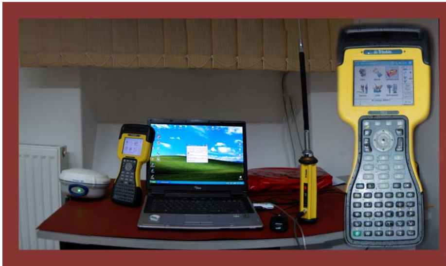
Fig. 1. The equipment used in order to transmit differential data corrections
