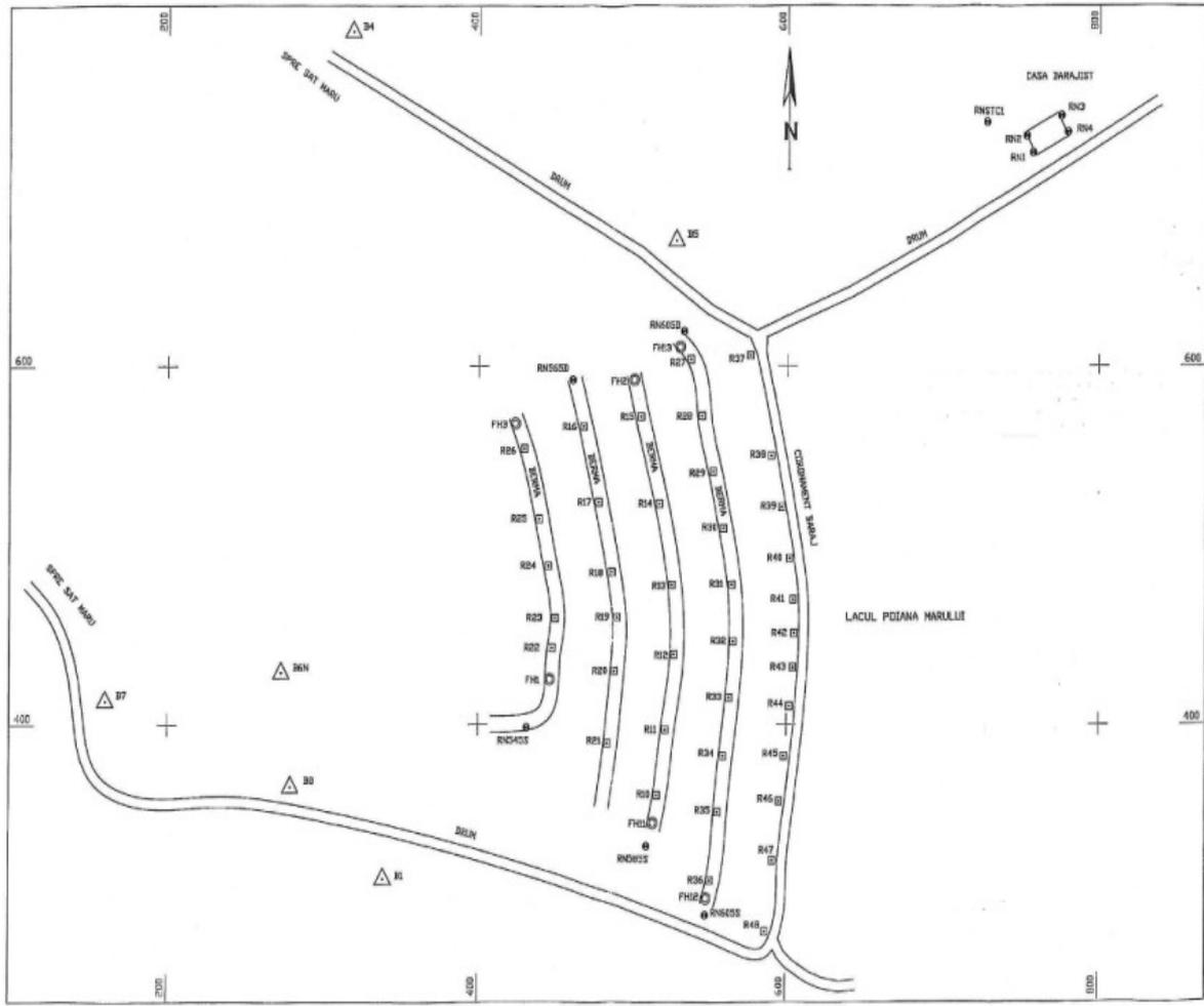
Figure 2. Sketch of tracking network Poiana Mărului dam3. Conclusions
