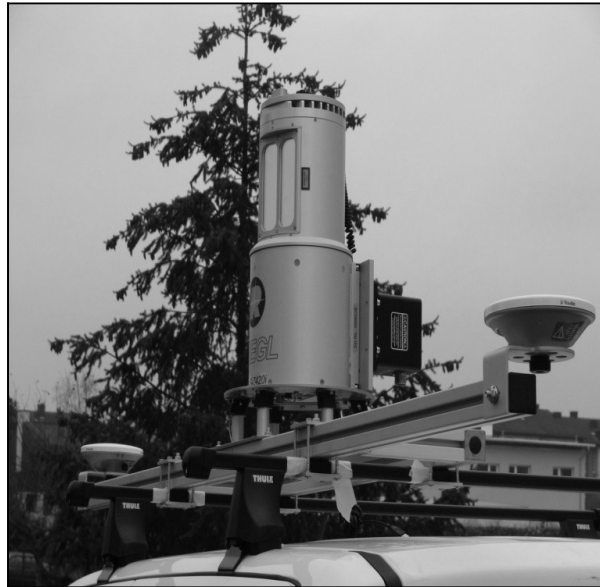
Fig. 6. – Mobile terrestrial laser scanning platform developed by S.C. C-TECH S.R.L.
