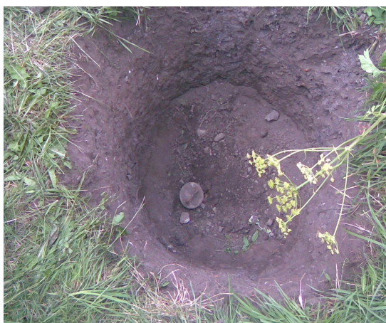
Fig.2 Leveling deep ground marker
