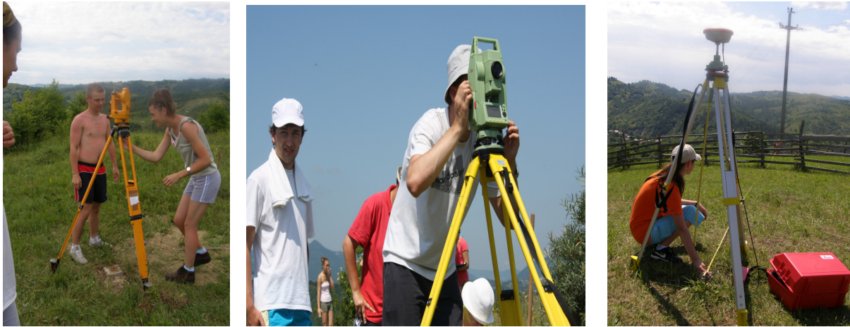
Fig.7 Classic and modern geodetic observations (triangulation, trilateration and GNSS)
