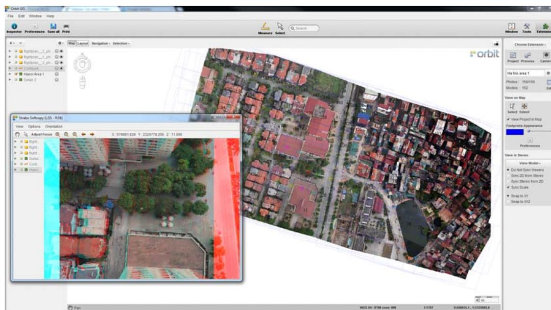
Fig. 2. Combining UAV 2D aerial images with 3D images in the same photogrammetry-GIS package (city project Hanoi, Vietnam 2011)
