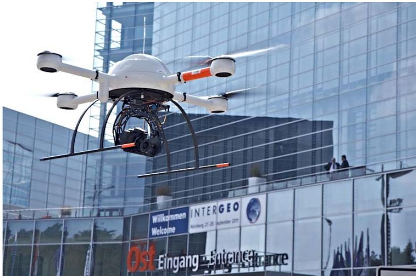
Fig. 6. the Microdrone MD4-1000 in action
