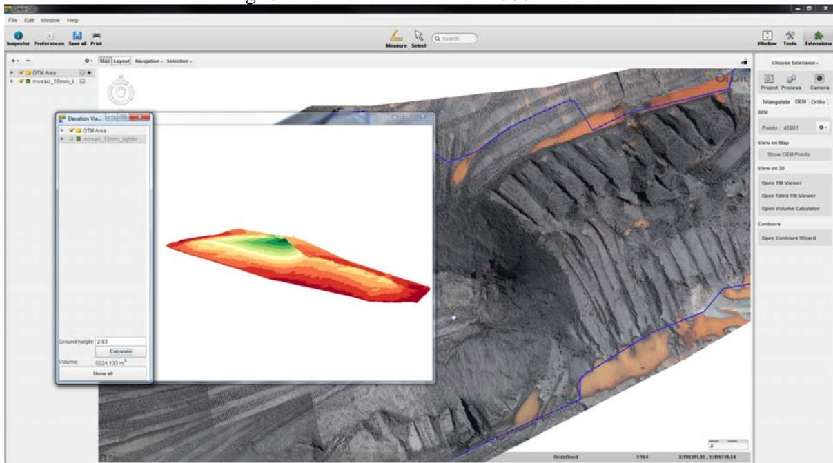
Fig. 7. The resulting 3D model of the surface mine.
