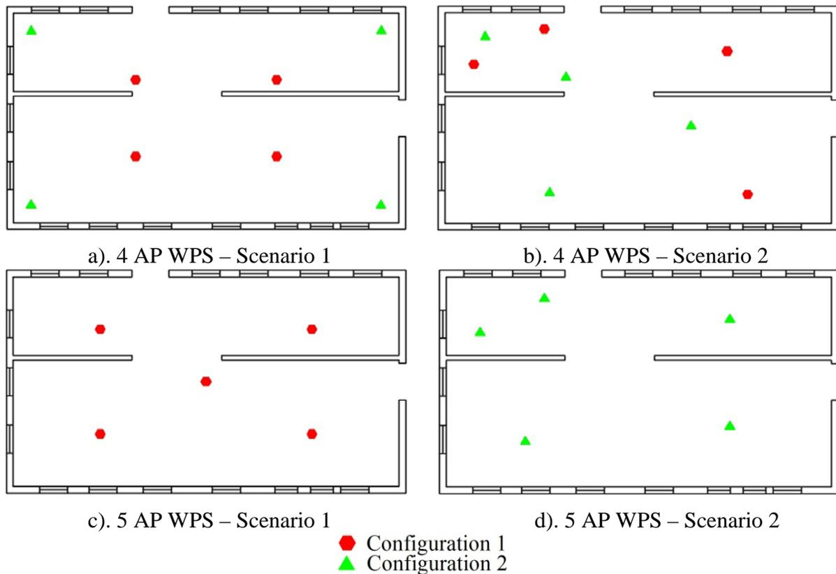
Fig. 3 – Simple Environment: 4 and 5 AP WLAN Configurations
