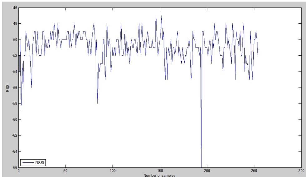
Fig. 6 – Received Signal Strength Indicator samples recorded from one Access Point
