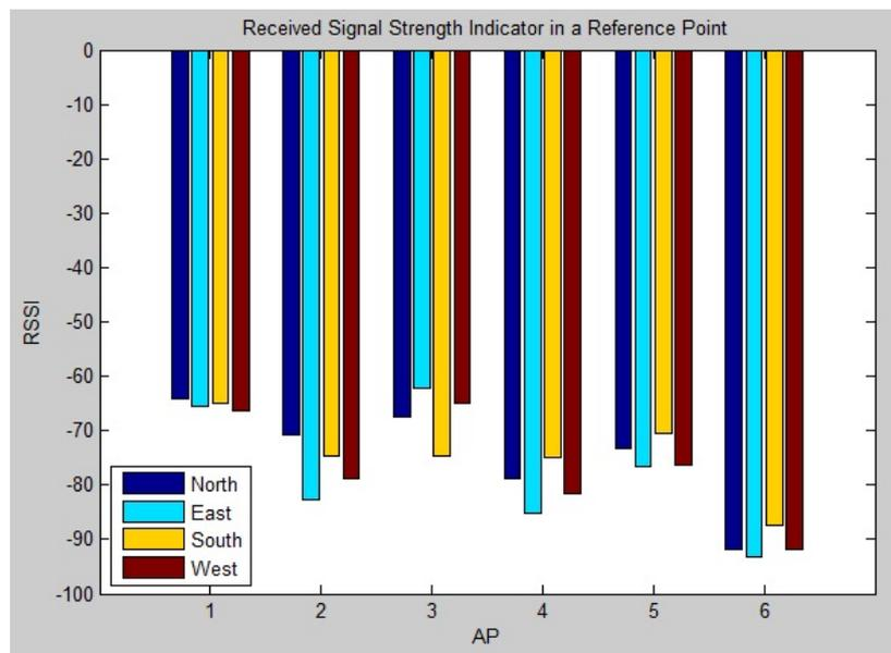
Fig. 7 – Received Signal Strength Indicator samples measured in one Reference Point on different headings
