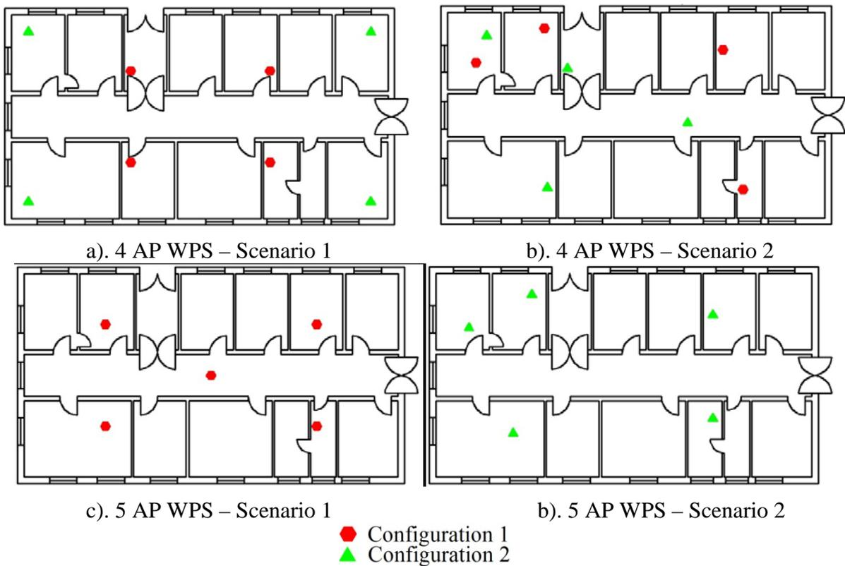
Fig. 4 – Complex Environment: 4 and 5 AP WLAN Configurations
