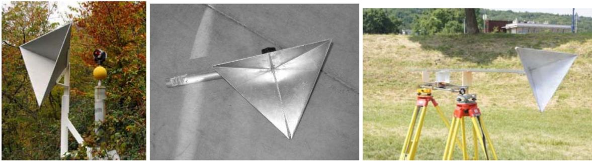
It is preferable that these points to be evenly distributed over the dam crest to estimate atmospheric corrections applied correctly to the GBInSAR system records, and thus for a better estimate of the possible deformations that occur. Theoretically, the proper selection of control points should eliminate any influence of the atmosphere, but if there are zones of highly differing weather conditions (e.g. low fog), the final result will be less accurate.
