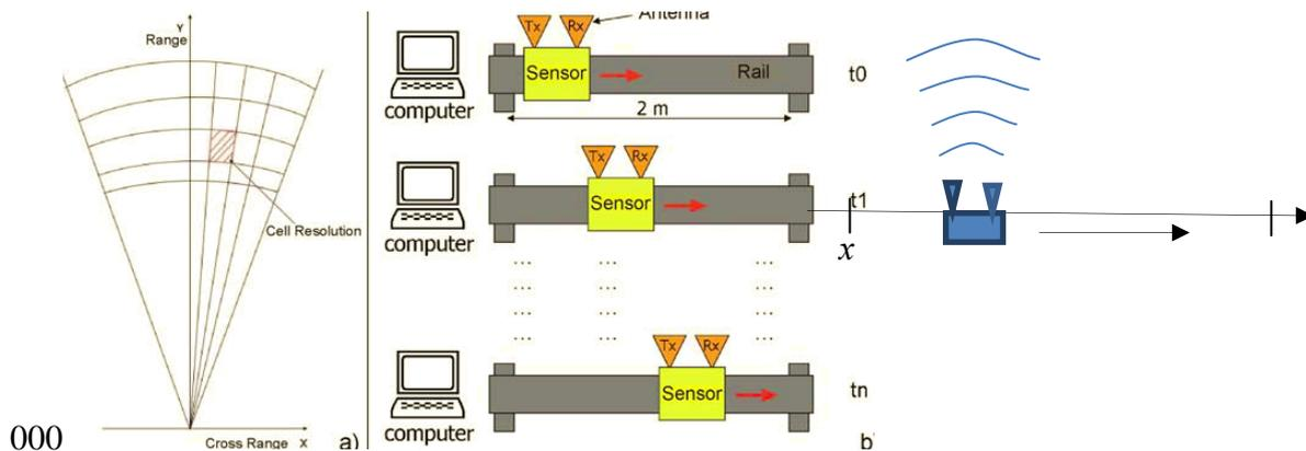
Analogously to pulse compression in range, the resolution in azimuth is obtained by compressing the range measurements in the cross-range direction (Hanssen, 2001). To obtain resolution in range a long pulse is compressed. In the cross-range direction a long acquisition time acquiring multiple range measurements is compressed into a single image considered captured at a same instant of time. Cross-range is defined as an angular resolution
