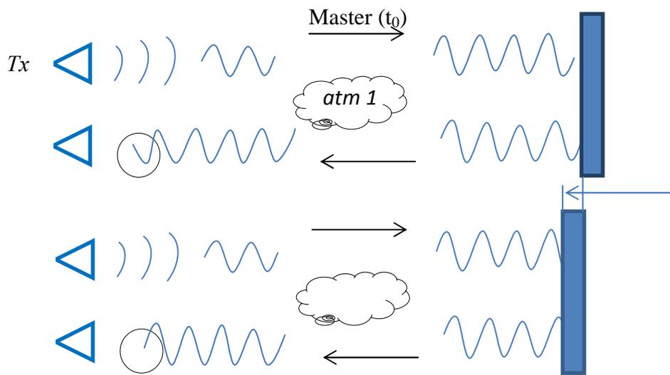
Since the images to be compared are acquired at different instants of time the atmospheric conditions must be considered. The variation of the diffraction index, due to temperature, humidity and pressure, causes a variation of the wavefront propagation velocity which may introduce an error in the range measurements.
