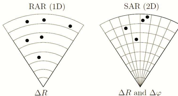
Resolution is defined as the minimal distance at which two distinct scatters of the same brightness can be uniquely discerned as a separate signal (Hanssen, 2001). To distinguish between objects at different distances a short pulse is used. A shorter pulse means a better resolution (Skolnik, 1990).
