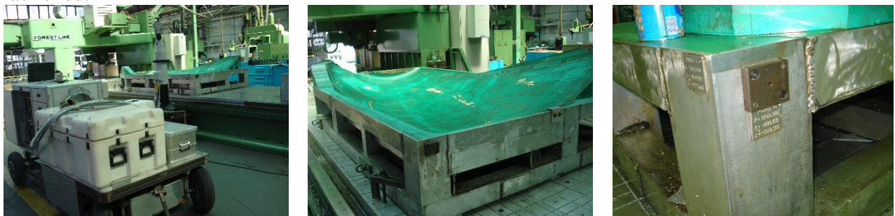
Fig 2.5. Laser tracker in measuring position. Atrape mounted on a cutter. Plates with coordinate in the system of the airplane which is on atrape
