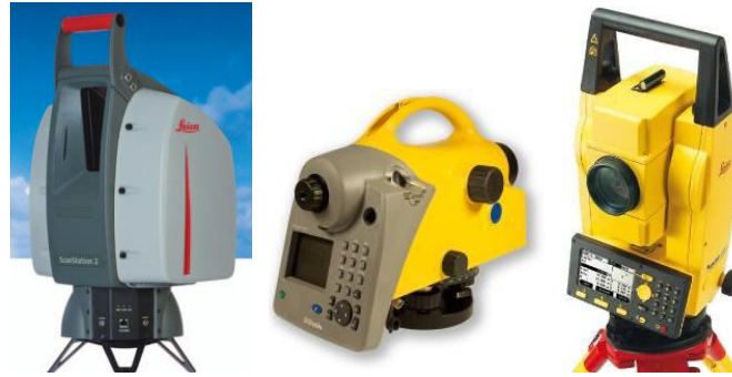
Fig. 2 – Equipment used for measurements (laser scanner, level, total station)
