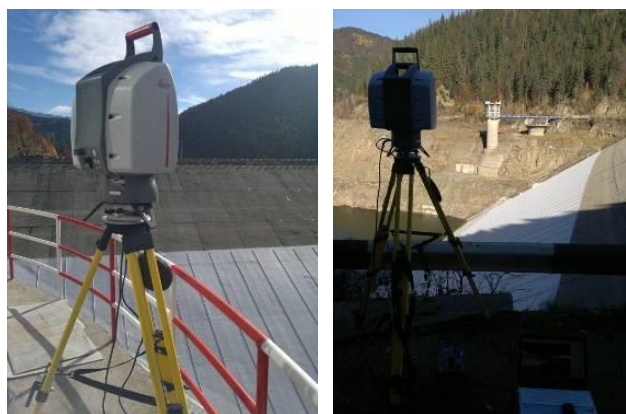
Fig. 4 – Measurements using laser scanner
