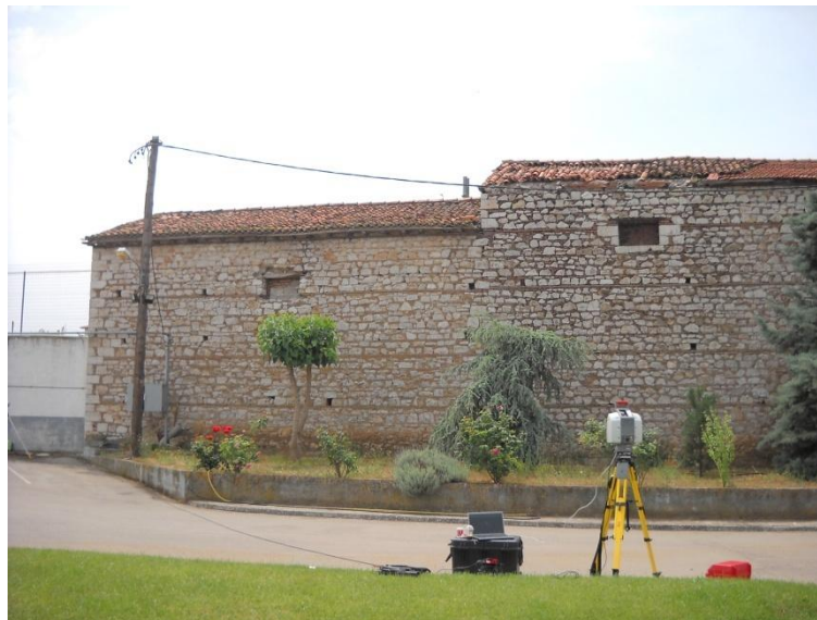
Figure 3: Leica ScanStation2 TLS during scanning process
