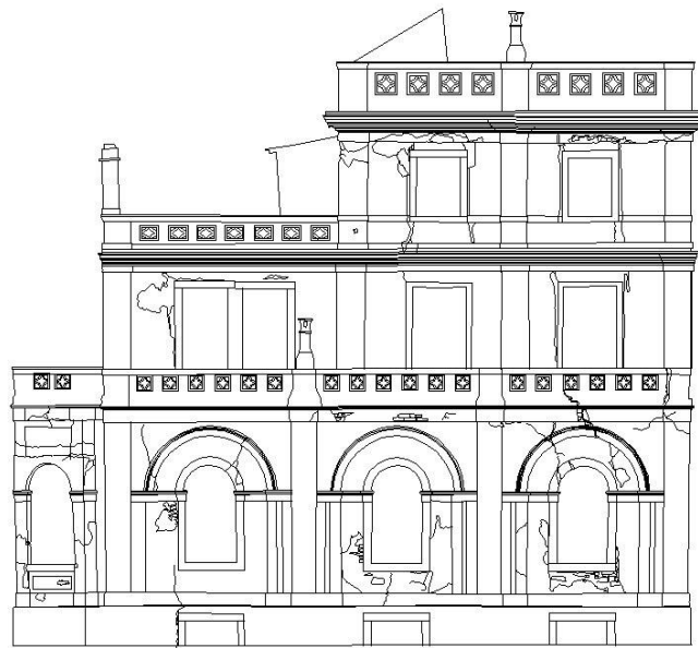
Figure 6: Vector drawing produced from photomosaic showing damages
