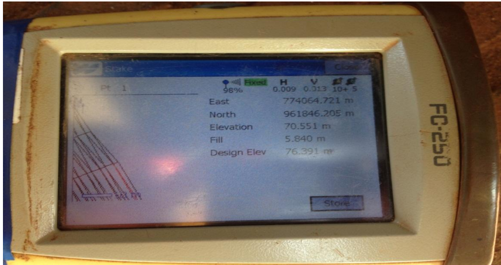
Fig. 10. Loading 3D models directly surveying instruments
