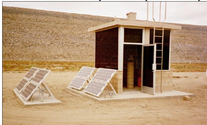
Fig. 6 Total stations supply with photovoltaic cells
