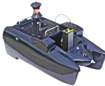
Fig. 2. Model Sonar Jet Boat with 360 deg Prism and Sonarmite Echo Sounder
