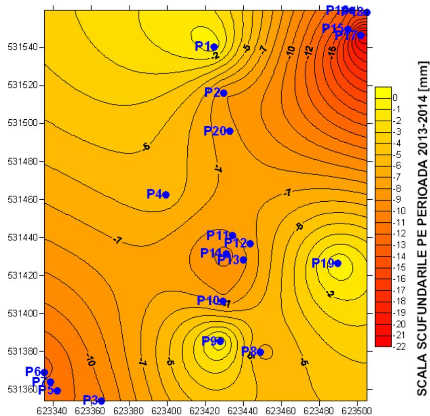
Fig. 2. Curves of Equal Immersion during 2013-2014
