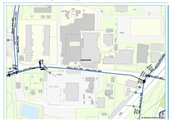
Fig. 4. Provited plan of water network
