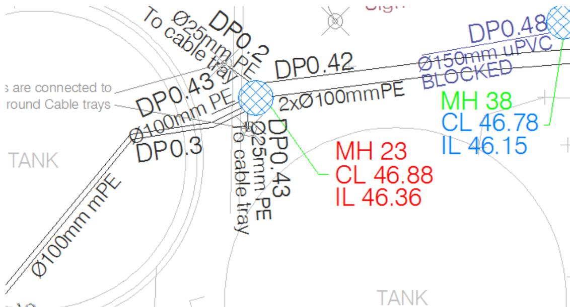
Fig. 6. Manhole details added manually using the form
