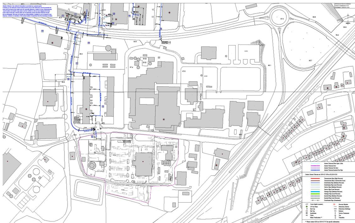
Fig. 2. Provided plan of gas ducts
