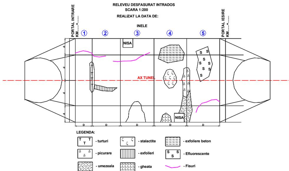
Fig. 5. The conducted mapping plan of the soffit
