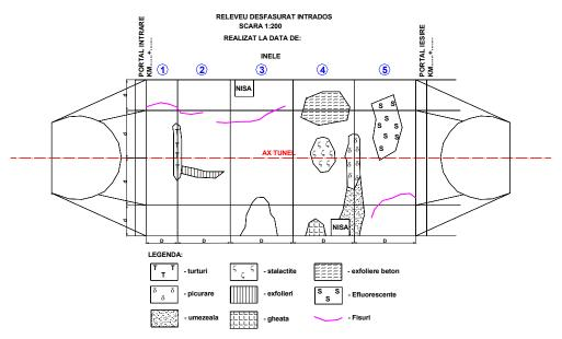
Fig. 5. The conducted mapping plan of the soffit
