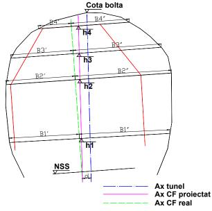
Fig. 6. Measurements of transverse surveys
