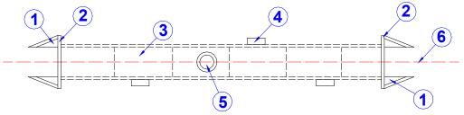
Fig. 2. Characteristic elements of tunnel 1 - wing, 2 – portal, 3 – ring, 4 – niche, 5 – ventilation shaft, 6 – tunnel axis
