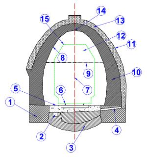
Fig. 3. Characteristic elements of tunnel
