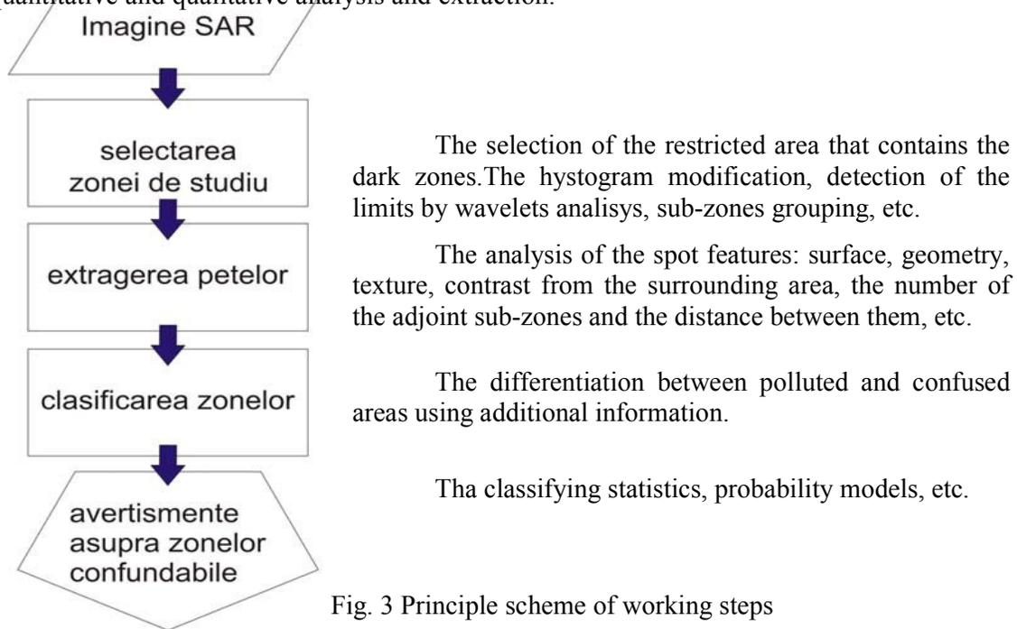
Fig. 3 Principle scheme of working steps
