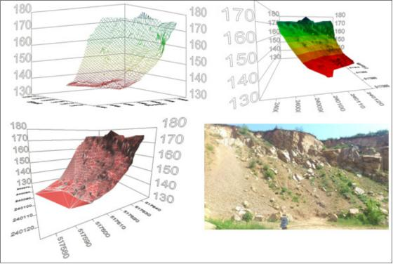
Fig.7. The real surface and its DTM
