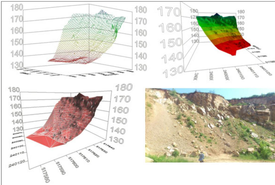
Fig.7. The real surface and its DTM
