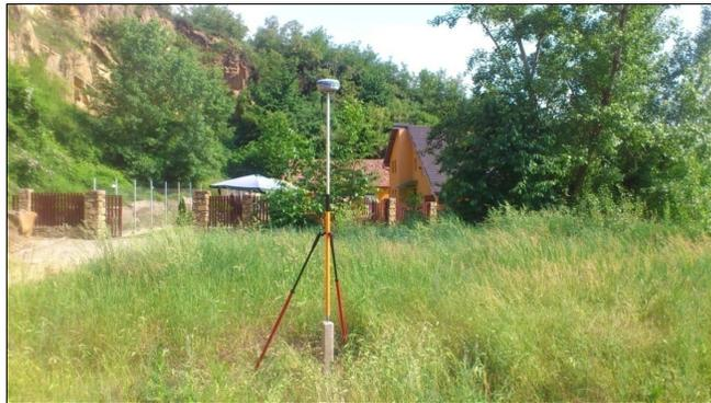
Fig.2. Determining the first station point coordinates
