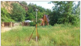
Fig.2. Determining the first station point coordinates
