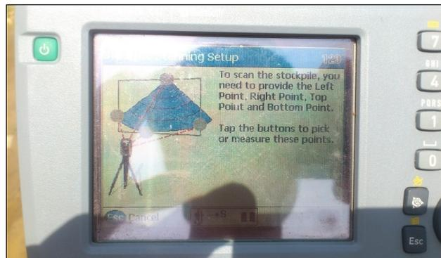
Fig.4. The terrain surface' limits establishing
