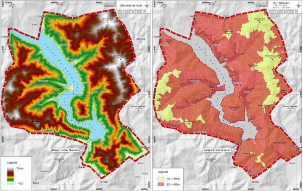
Fig. 6. Height above the lower reservoir
