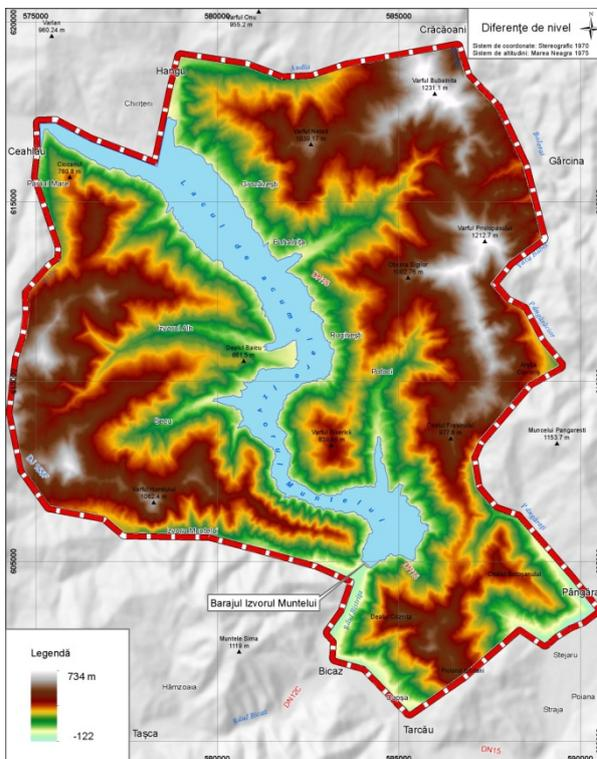
Fig. 6. Height above the lower reservoir
