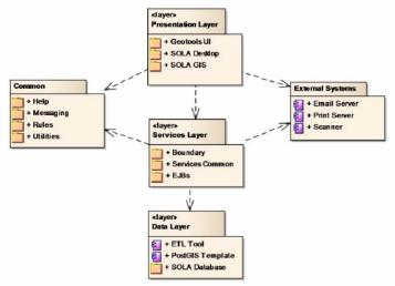
Figure 11 - SOLA package overview (SOLA Software Architecture Document, 2011)
