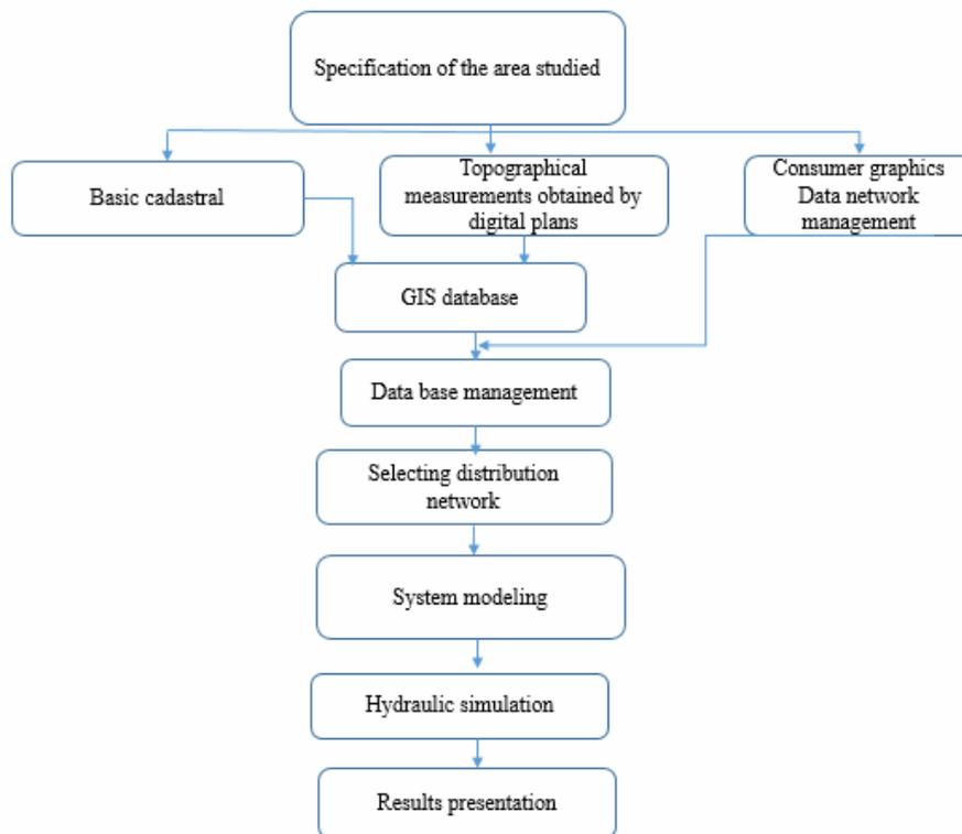
Fig.1. The diagram of the modelling of the studied zone
