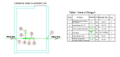
Fig.3. The hydraulic scheme
