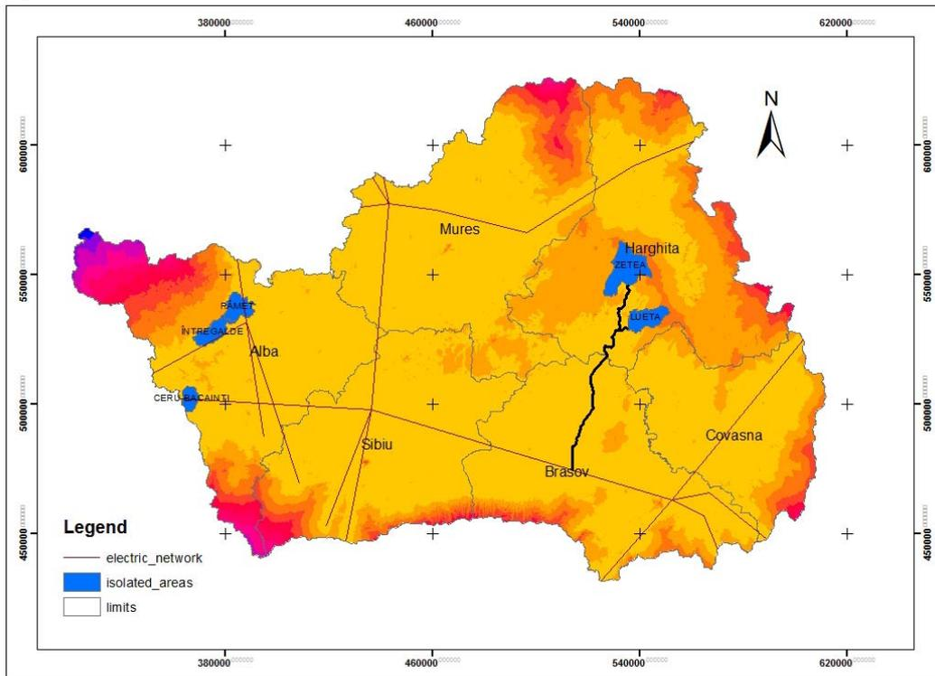
Fig. 2.5. Cost path for electric network map
