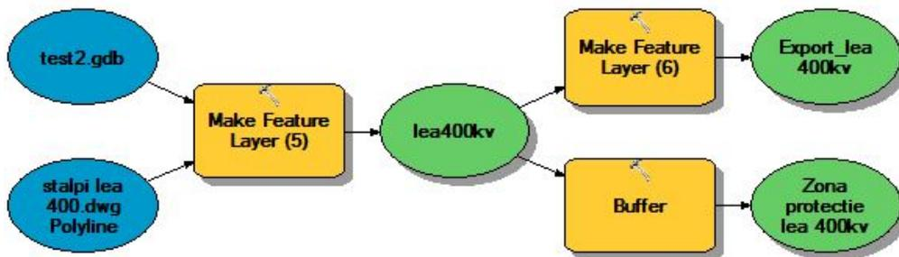
Fig. 6. ModelBuilder for creating protection zone of overhead power lines
