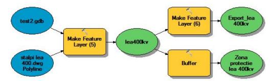
Fig. 6. ModelBuilder for creating protection zone of overhead power lines
