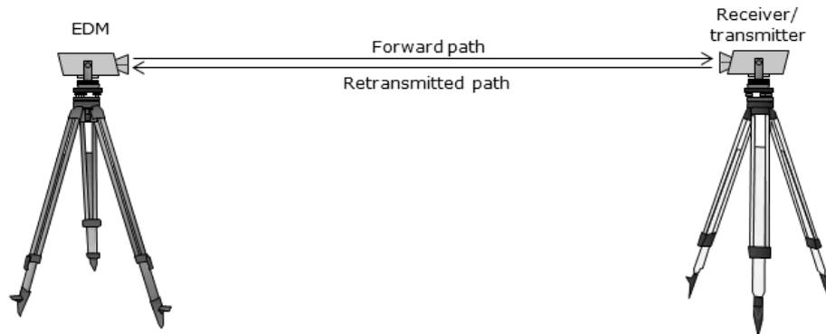
Fig. 1 EDM<sup>1</sup> Instrument [8]
