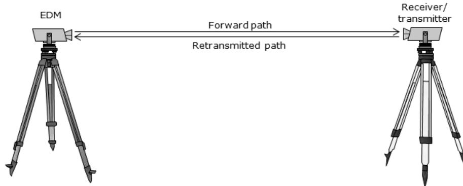
Fig. 1 EDM<sup>1</sup> Instrument [8]
