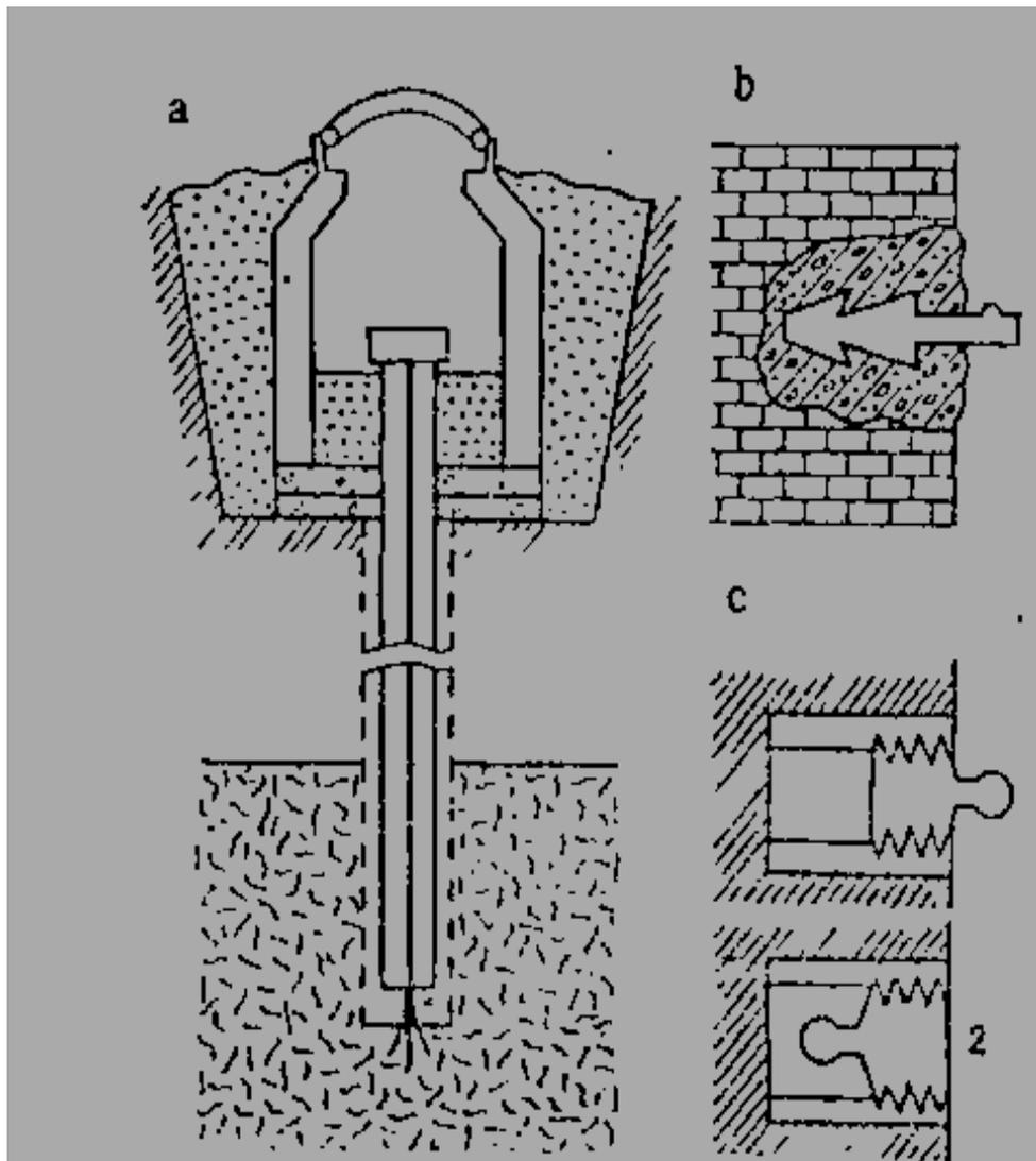
Fig. 1. Signals Fixing points for making observations on settlements bridges
