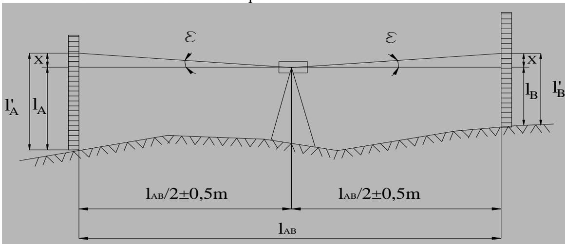
Fig. 4 Collimation error in leveling influence of geometric means
