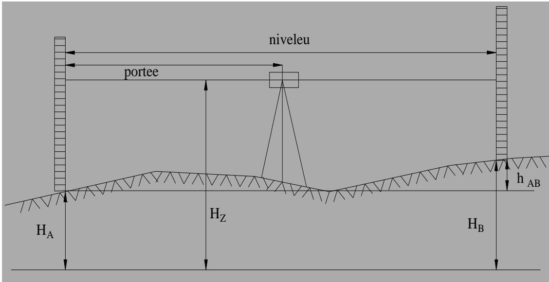
Fig. 3 Geometric leveling method
