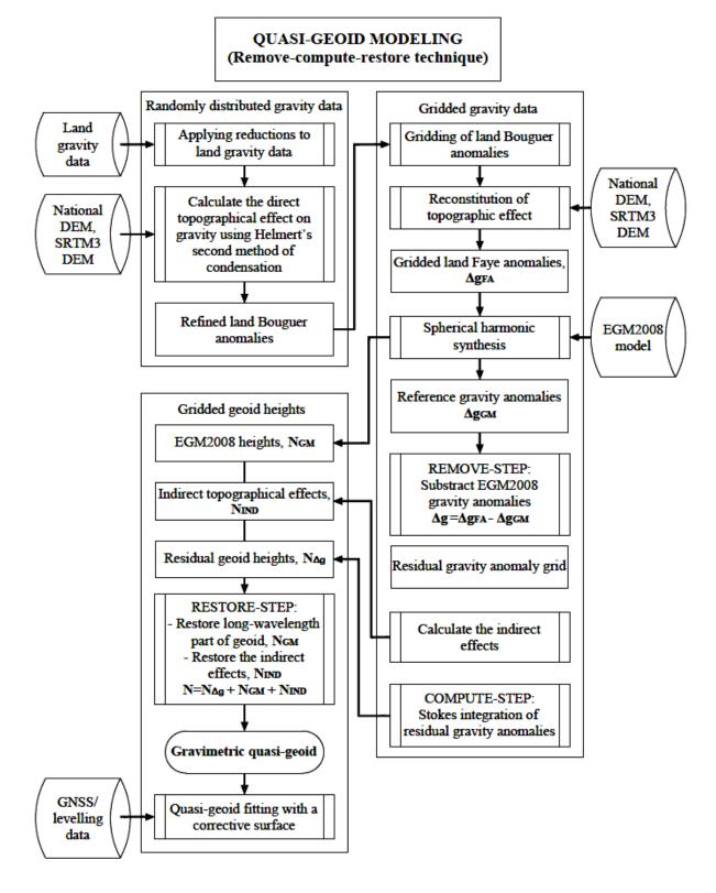
Fig. 3. Logical Flowchart of a quasigeoid model
