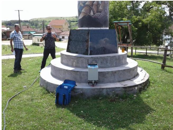
Fig. 2. Performing gravimetric measurements in a new point of a loop
