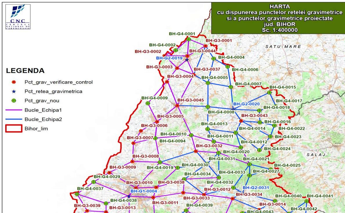
Fig. 1. The layout of the gravimetric points in the pilot project from Bihor County
