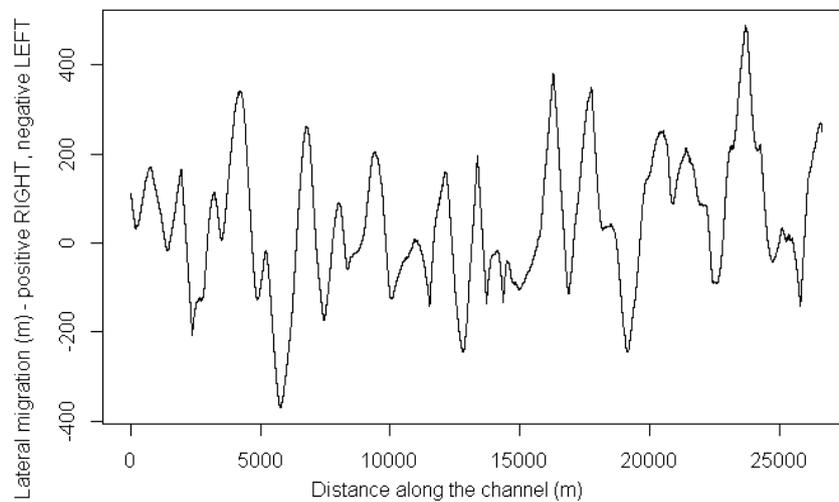
Fig. 8. The lateral migration rates of Prut river channel between 1893 and 2016
