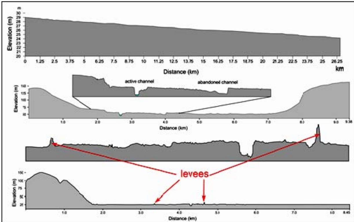
Fig. 2. Topographic profiles in the Prut River floodplain and channel: longitudinal profile (above), transversal section trough unconstricted channel (middle), and transversal section trough constricted channel between embankments (bottom)
