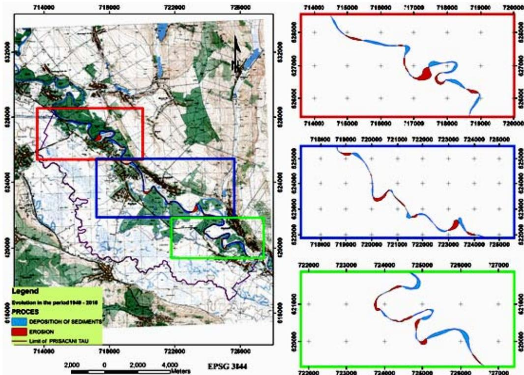
Fig. 6. The erosion and deposition areas of Prut river channel between 1949 and 2016
