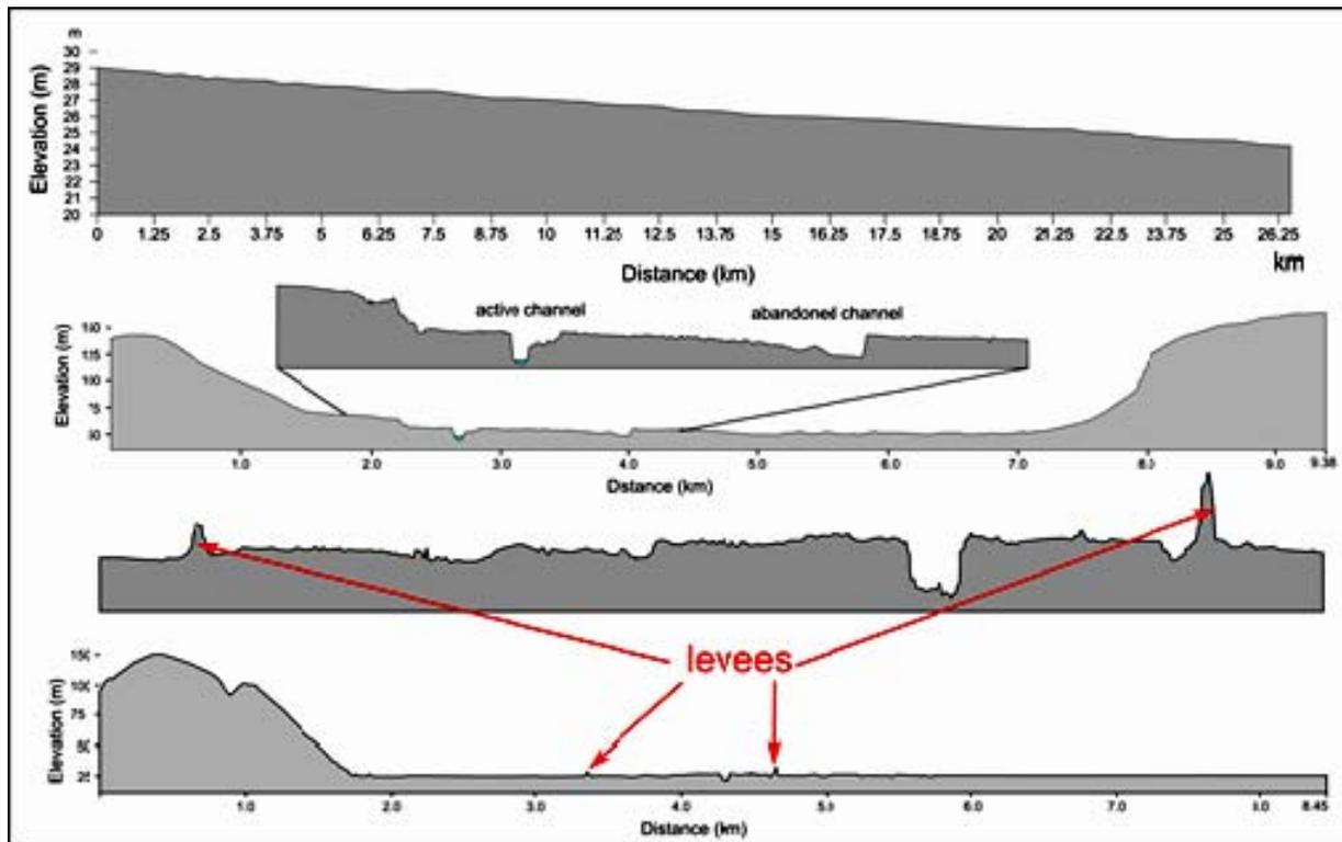
Fig. 2. Topographic profiles in the Prut River floodplain and channel: longitudinal profile (above), transversal section trough unstricted channel (middle), and transversal section trough constricted channel between embankments (bottom)
