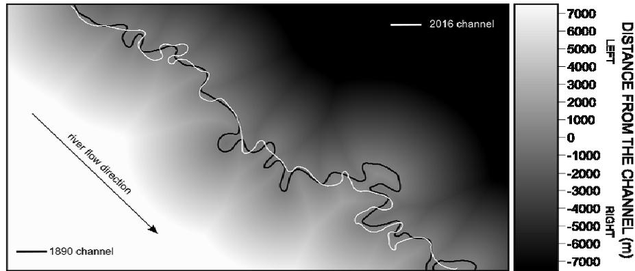
Fig. 5. The raster approach for estimating river channel lateral migration rates
