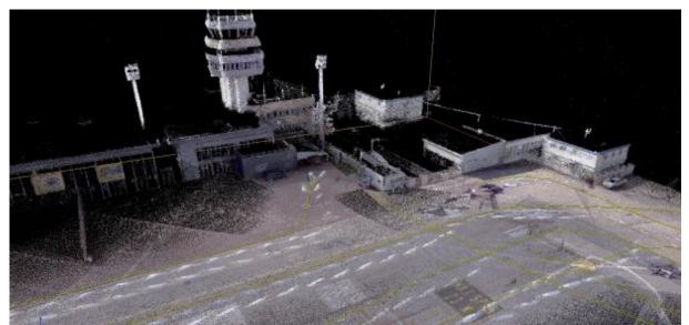
Fig. 6 Perspective view of the LiDAR processed points - airport main tower
