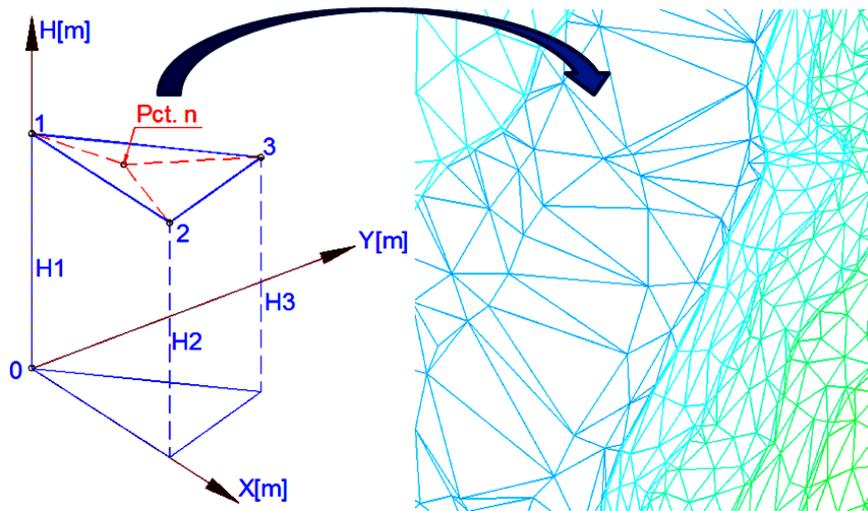
Figure 3 – The interpolation method of the H elevation for a point n in TIN
