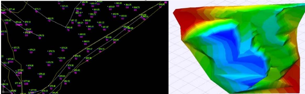
Figure 6 - a) G.N.S.S. measurements for determining D.T.M.
