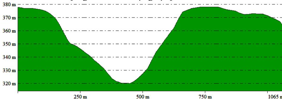
Figure 4 – Product resulted from the exploitation of the digital terrain model, transvere profile viewing a major river bed
