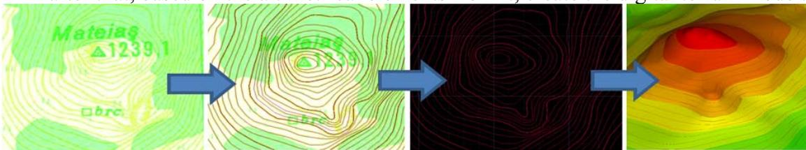
Figure 2 - Obtaining digital terrain model from old cartographic source, raster-vector conversion and subsequent creation of digital terrain model
