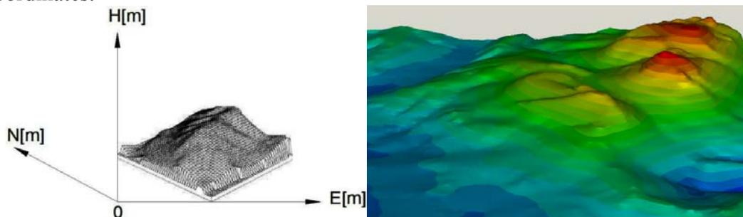
Figure 1 – a) Digital terrain model within a 3D coordinates system –  $N$ ,  $E$ ,  $H$
