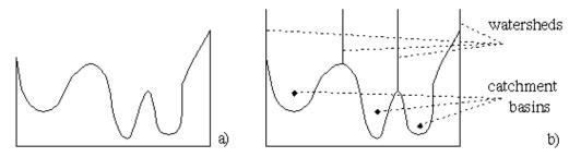
Fig. 3. a) Gray level profile of image data. b) Watershed segmentation – local minima of gray level (altitude) yield catchments basins, local maxima define the watershed lines.
