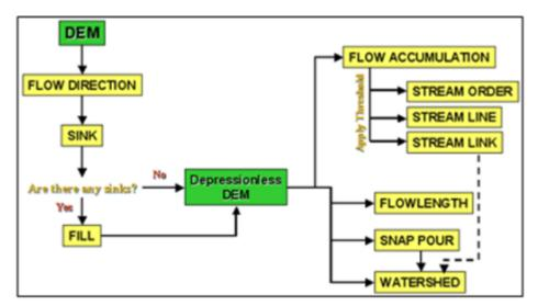
Fig. 2. The process of extracting hydrological information
