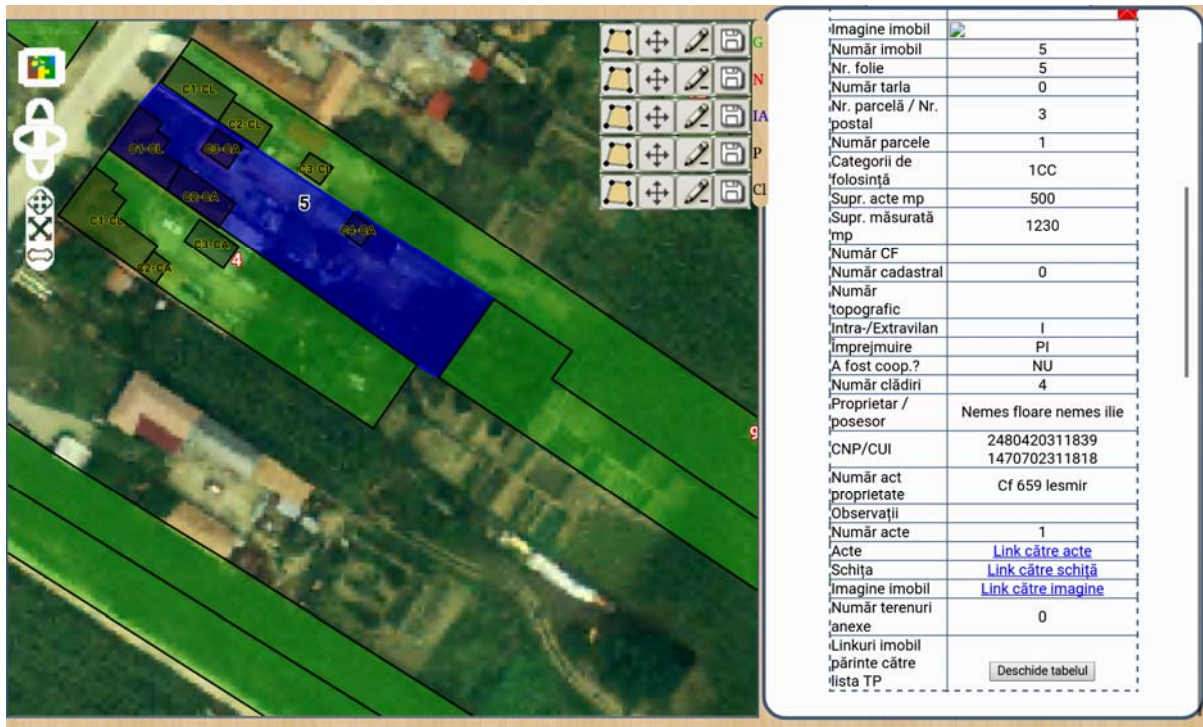
Fig. 8: After activating the selection mode, the user clicks on a plot or building and sees the information attached, besides the links toward the attached documents, sketch, and plot image.
