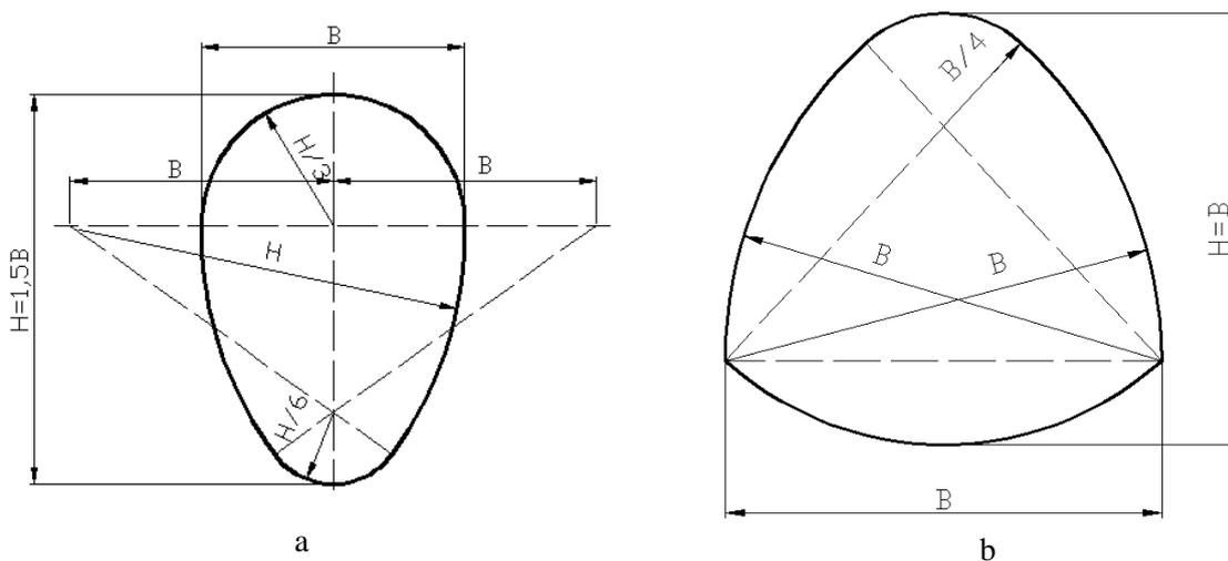
Fig. 2. Profile sewer visitable collectors standardized; a - kind ovoid; b - semi-elliptical bell.
