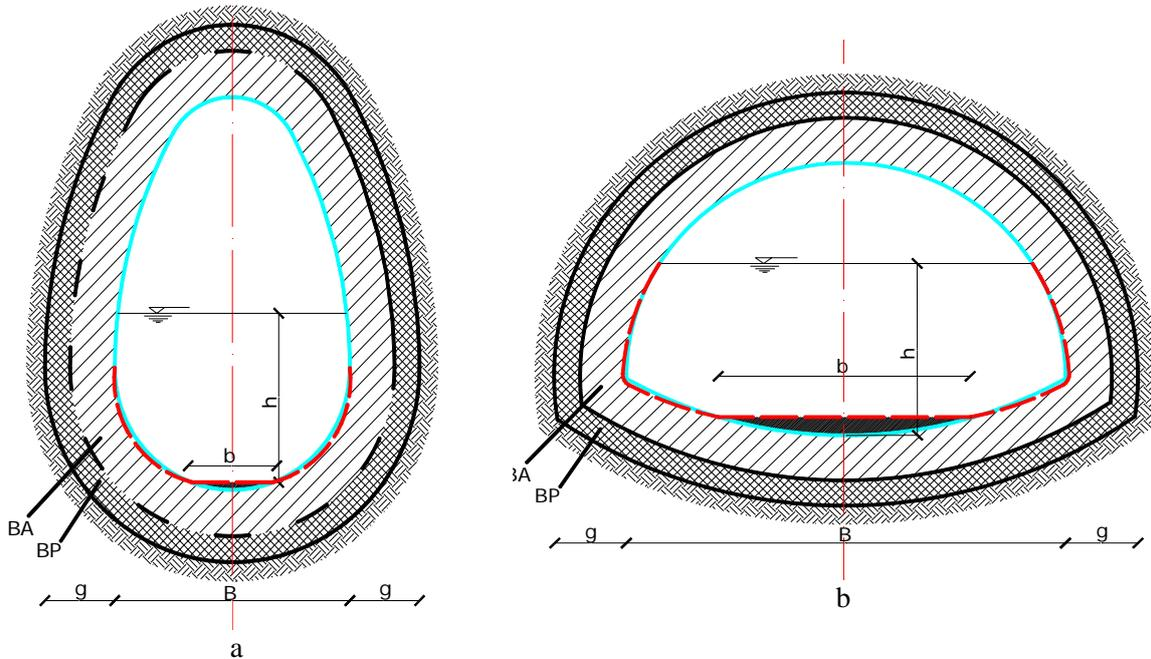
Fig. 3. Profile of the sewer visitable collectors changed (green line-formatted geometric initial red line - as amended (polycentric)); a – type ovoid; b – type circular bell.
