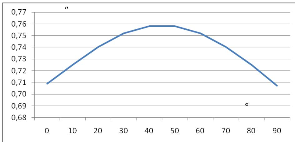
Fig. 6. The influence of deflection of vertical components on geodetic vertical angles
