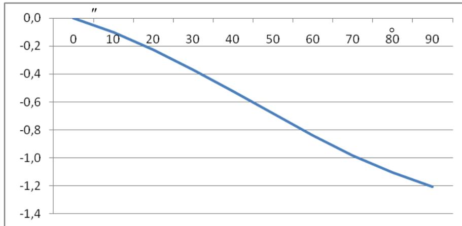
Fig. 5. The influence of deflection of vertical components on geodetic azimuths
