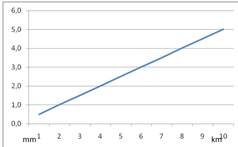
Fig. 7. The influence of deflection of vertical components on distances
