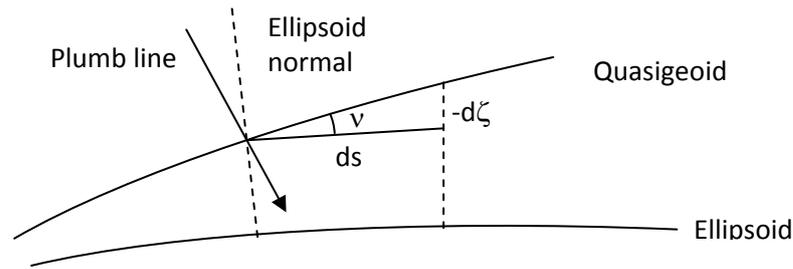
Fig. 2. Geometrical relationship between quasigeoid height and DoV
