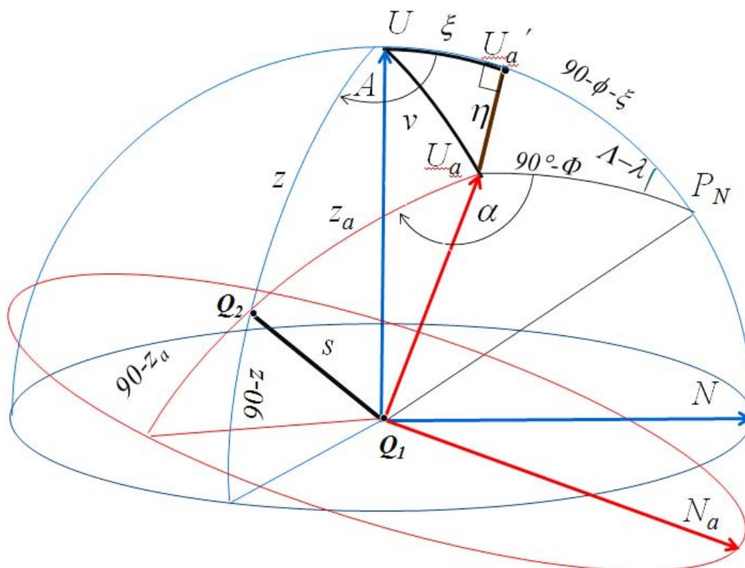
Fig. 4. Astronomical topocentric and geodetic topocentric systems of coordinates
