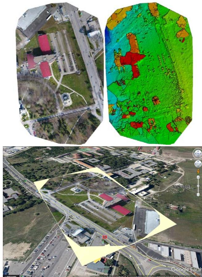
Fig. 9. The resulted Orthophotoplan (WGS 84), digital terrain model and the Google Earth view
