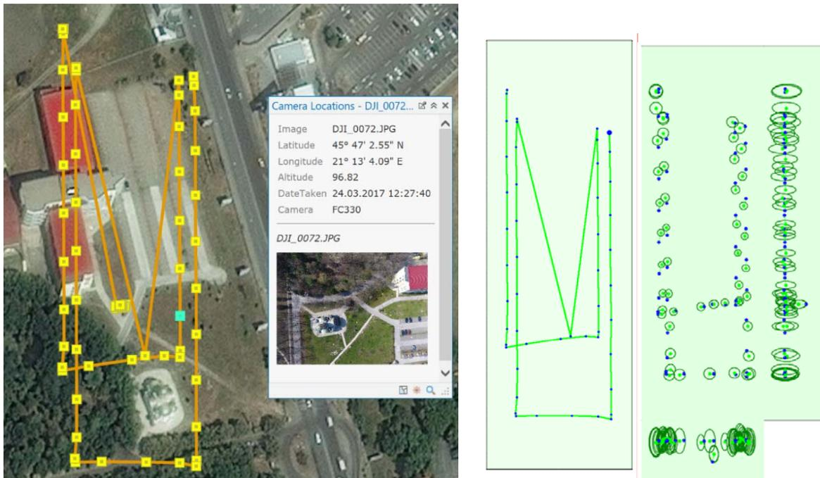
Fig. 8. The GPS position of the images
