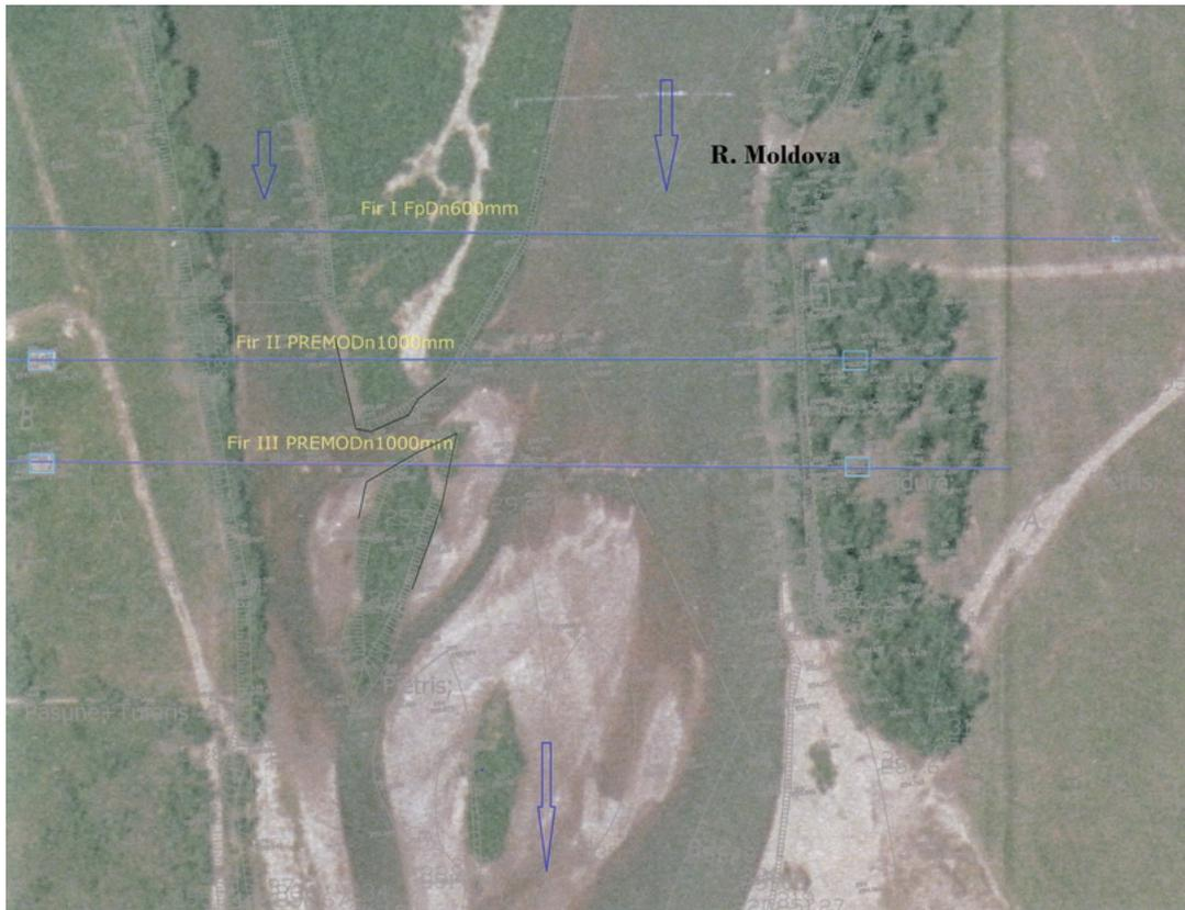
Fig. 1. Ortofotoplan with the location of hydrotechnical works on the Moldova River
