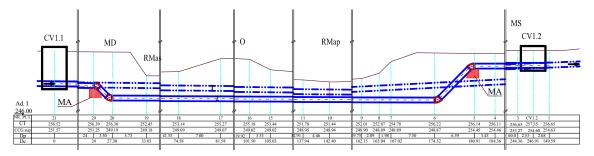
Fig. 8. The longitudinal section of AdI adduction pipe undercross: discontinued line - pipeline executed in 1911: continuous line - pipeline designed in 2012; CV1.1 and CV1.2 - camps with taps executed in 2012.
