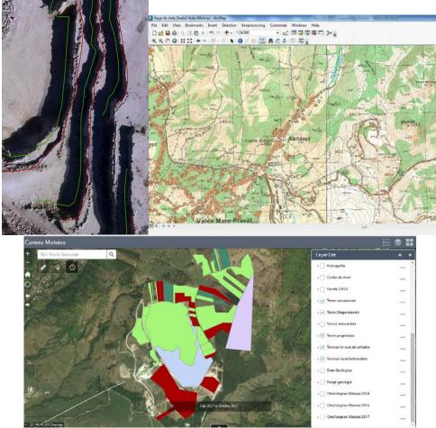
Fig. 3. View from the GIS database: up left orthophotomap mosaic with 50mm pixel resolution; up right Topographic map scale 1: 25000; bottom center-real estate informations
