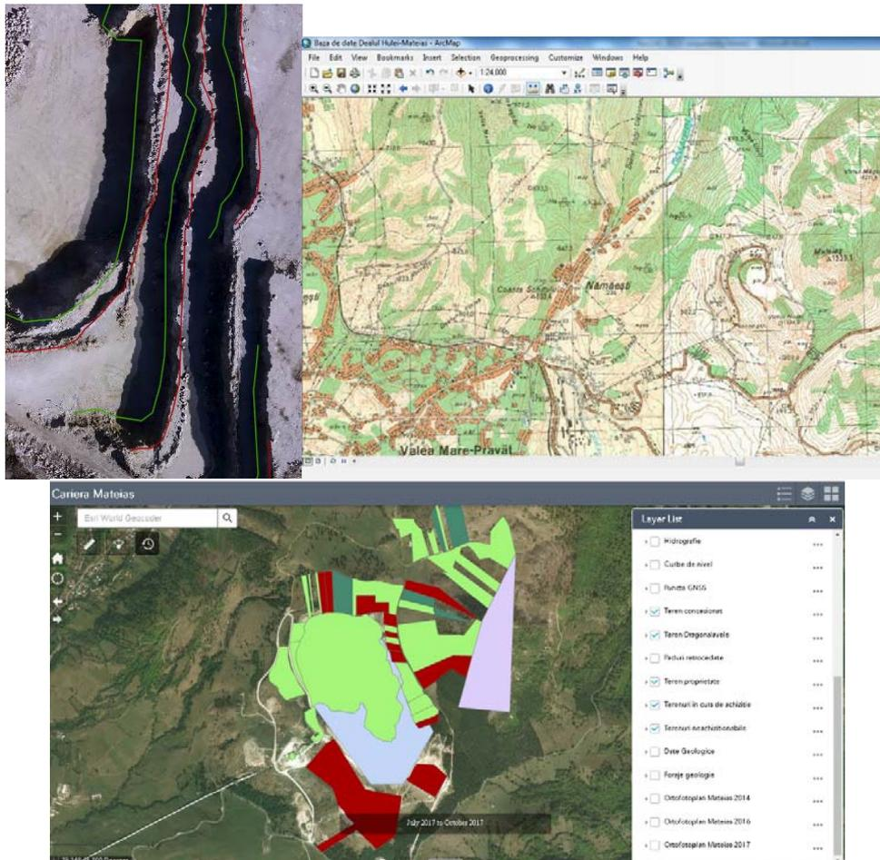
Fig. 3. View from the GIS database: up left orthophotomosaic with 50mm pixel resolution; up right Topographic map scale 1: 25000; bottom center-real estate informations
