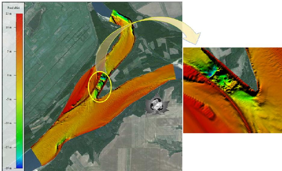
Fig. 10. The bathymetric model exported from the *Delft3D* program. Detail the Bala branch
