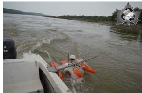
Fig. 3. *RiverRay* bathymetrical system
