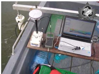
Fig. 2. *River Surveyor M9* bathymetrical system
