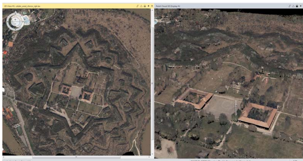
Fig. 12. RGB encoded point cloud for Arad Fortress (2D and 3D view)
