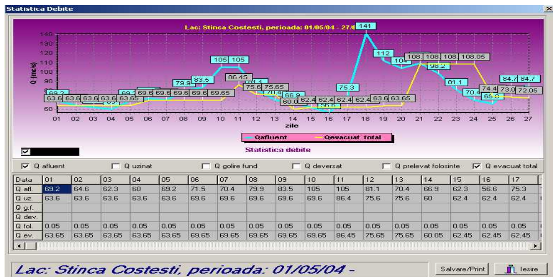
Fig.2. Variation of the daily affluent, turbine and evacuation flows at the Stanca-Costesti node
